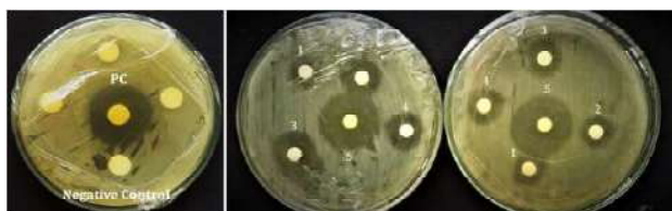
Fig. 6 : Anti bacterial activity of synthesized CNPs against phytopathogenic strain Xanthomonas oryzae duplicates of different concentration after 24 h of incubation. 1-2mg/ml, 2-4mg/ml, 3- 6mg/ml, 4-8mg/ml and 5-positive control (PC) (Tetracycline), different concentration of CNPs used to examine the most effective CNPs concentration for antimicrobial activity
