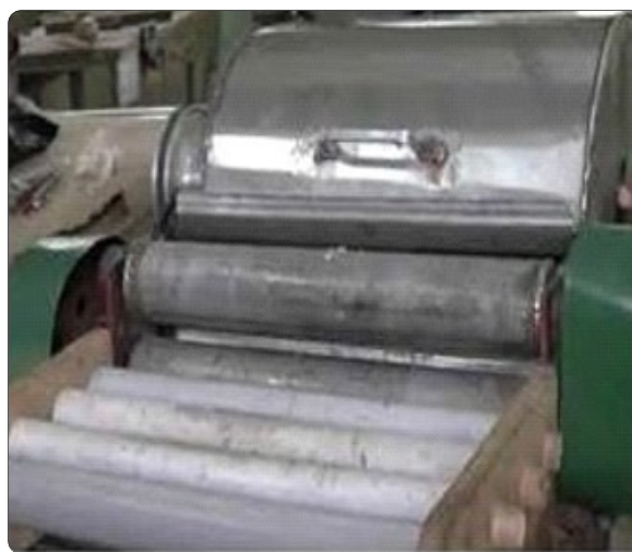
b). Enset sheave decorticator machine
