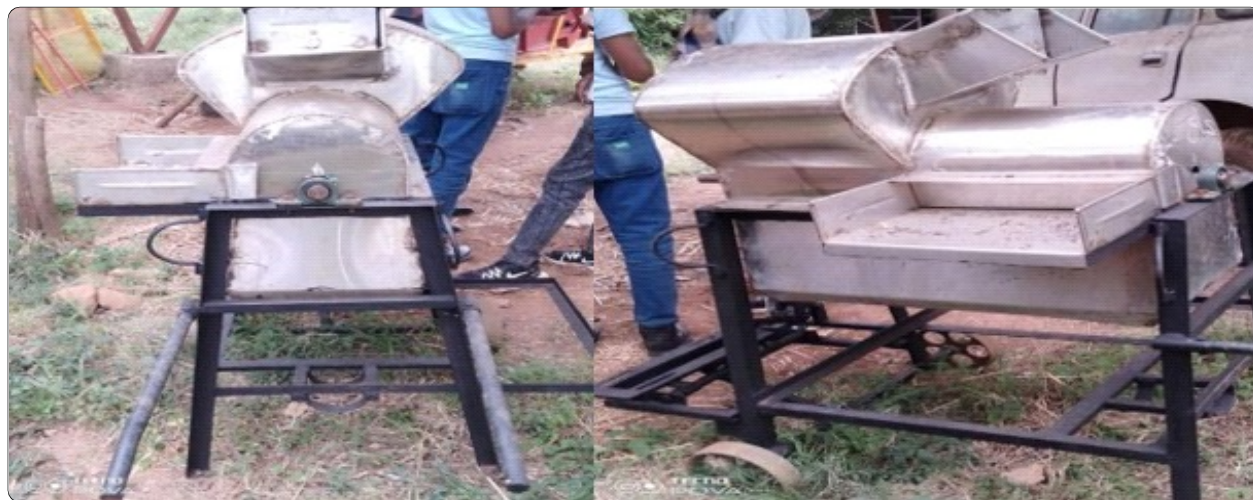
Fig. 5(c) : An integrated enset processing machine available at BAERC
